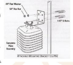
wrap around the pipe. Secure the TRH-6200 to the pipe.
